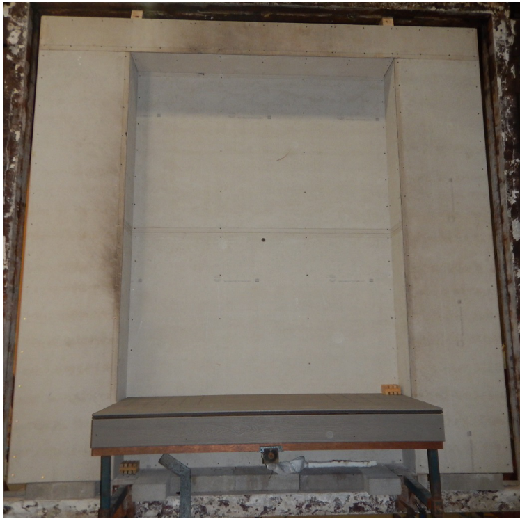
Figure A1 – Exposed face of specimen before commencement of the test.
